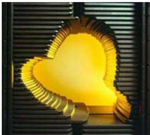
Fig. 2. The leaf pairs of a multileaf collimator
